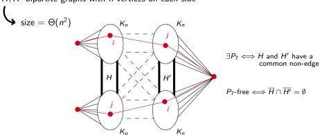
In the certificates,  $\Theta(n^2)$  bits of information have to be transmitted through O(n) vertices
