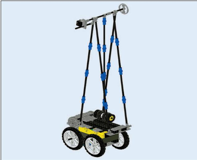
**Figure 1.** The cart and pendulum system. This view is generated using the LEGO design program Ldraw. The corresponding parts lists are given in Tables 1 and 2. The large yellow brick contains the microprocessor, and has three sensor inputs and three actuator outputs. The pendulum is suspended from a triangulated gantry attached to the cart. More detail appears in Figure 4.
