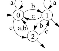
FIGURE 1. The minimal automaton of a language  $L$ .
