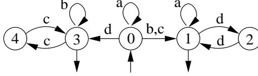
FIGURE 3. The minimal automaton of a language  $L$ .
