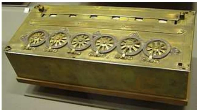
The first calculator to have a controlled carry mechanism which allowed for an effective propagation of multiple carries.
