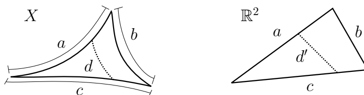
Fig. 3: A chord in a triangle in X , and the corresponding chord in the comparison triangle in the plane. The triangle in X is thin if d \leq d' for all such chords.
