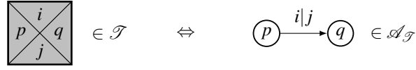
Fig. 10.5 The transducer \mathcal{A}_{\mathcal{T}} associated with a Wang tileset \mathcal{T} according to Culik-Kari.
