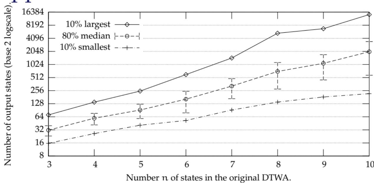
Average number of states in the 10 smallest, the 10 largest, and the 80 median accessible bottom-up tree automata obtained from transforming 100 2-letter DTWAs with  $n$  states
