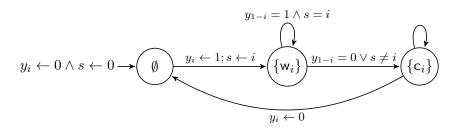
2. The best way to see that mutual exclusion holds is to construct the "low level" transition system and check that no state with both  $c_0$  and  $c_1$  holding at the same time is accessible. Here is half of it:
