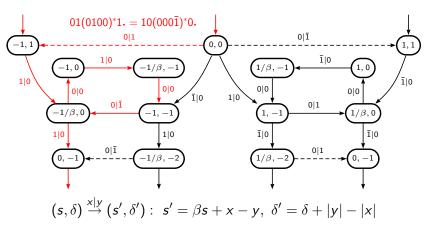
For  $\beta = \frac{1+\sqrt{5}}{2}$ , all signed  $\beta$ -expansions of minimal weight are given by the following automaton, where all states are terminal, and by the following branching transformation.
