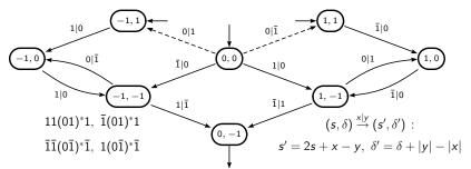
All expansions of minimal weight (in base 2) are recognized by the following automaton, where all states are terminal.
