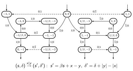
The strictly  $\beta$ -heavy words are the inputs of the following transducer. The outputs are corresponding lighter words (if the path is completed by dashed arrows such that it runs from (0,0) to (0,-1)).
