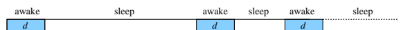
Fig. 4. Illustrating a free sensor that alternates between awake periods of fixed length d and sleep intervals of arbitrary lengths.
